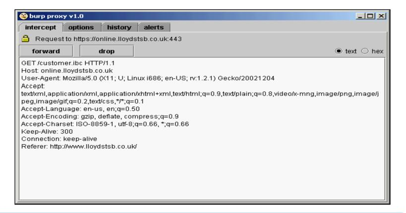
Burp proxy operates as a man-in-the-middle between the end browser and the target web server, and allows the attacker to intercept, inspect, and modify the raw traffic passing in both directions
